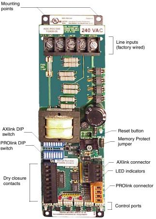
FIG. 1 RDC-PDC control card
